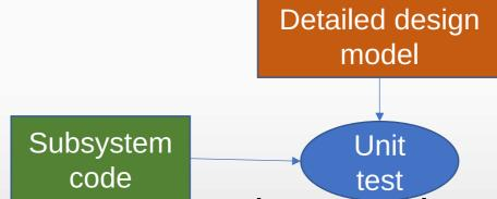
Goal: Confirm that subsystem is correctly coded and carries out the intended functionalities
